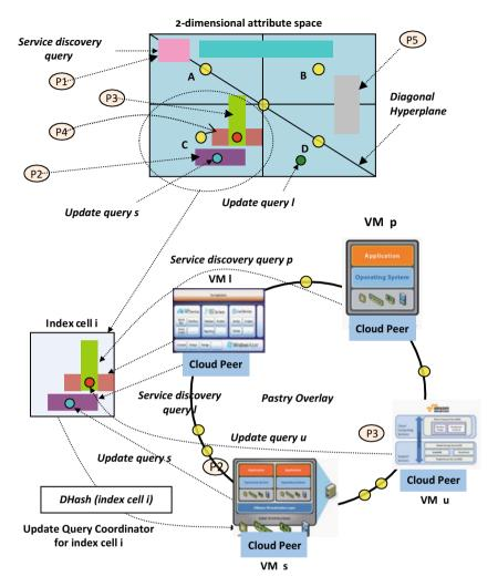
**Fig. 12.3** Co-ordinated provisioning across VM instances: multidimensional service provisioning requests {P1, P2, P3, P4}, index cell control points {A, B, C, D}, multidimensional update queries {1, s}, and some of the spatial hashing to the Pastry overlay, i.e. the multidimensional (spatial) coordinate values of a cell's control point is used as the Pastry key. For this figure,  $f_{min} = 2$ , dim = 2
