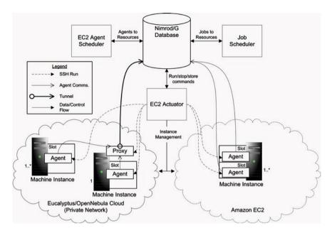
Fig. 13.1 EC2 extension architecture
