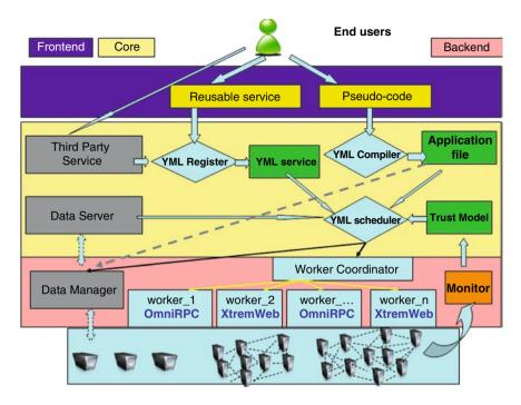
Fig. 9.5 Core part of YML-PC
