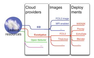
Fig. 11.4 The image catalogue hierarchical architecture
