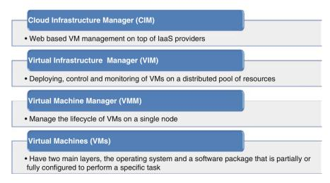
Fig. 1.2 Different layers of VM management tools and technologies
