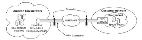
Fig. 10.8 Example of a simple Cloud seeding scenario
