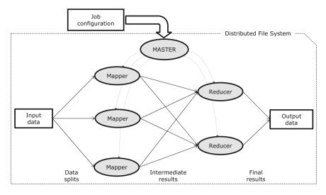
Fig. 7.1 Execution phases in a generic MapReduce application
