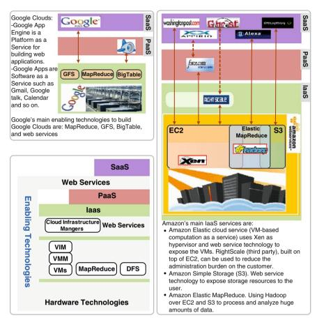
Fig. 1.1 Cloud services and enabling technologies, using Amazon and Google systems as examples
